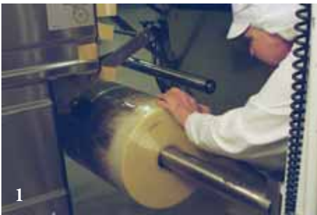
1-2. Changing rolls in packaging machines is carried out swiftly and safely with the V-block (right) and boom (above). The V-block is detachable so that the platform can be used for other chores in between changes.
